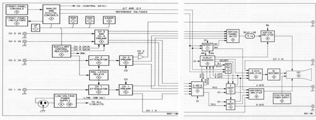
Figure 3-1. Block diagram.
