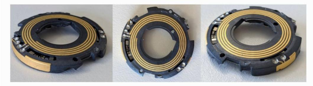
They are all etched onto a single piece of plastic using Laser Direct Structuring (LDS) and then soldered to the PCB around the edge. The NFC antenna also has a short trace on the other side of the plastic (connected with a via at each end) to return the inside end of the coil to the PCB.
