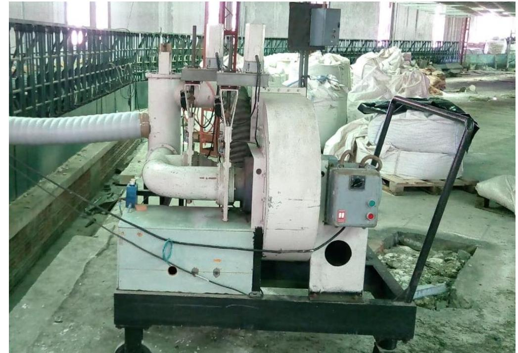
Air curtain turbine with damper setting facilities
